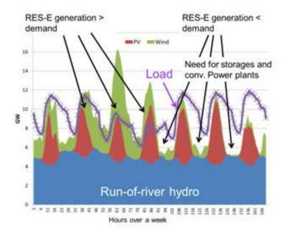
Performance of VR from wind, photovoltaics and run-of-river hydro plants over a week in summer on an hourly base in comparison to demand (Source: Haas [4])
