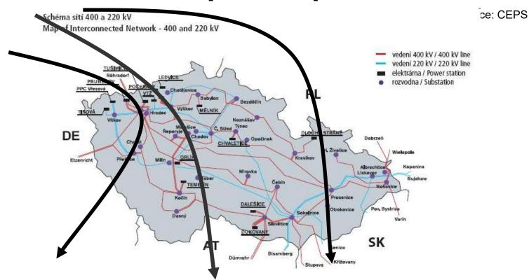
Problem: Loop flows from N. Germany to S. Germany and Austria, end of 2014: > 3400 MW from Germany to Austria
