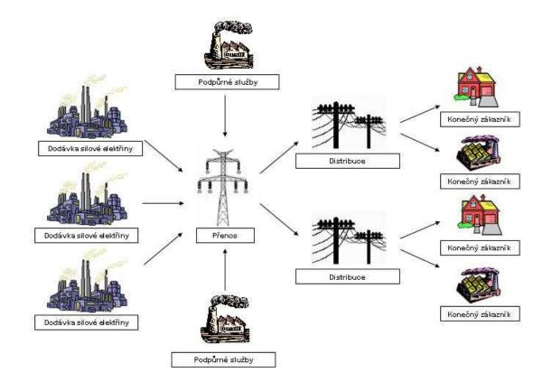
TS: 400 and 220 kV DS: 110, 35, 22 kV and 230/400 V
